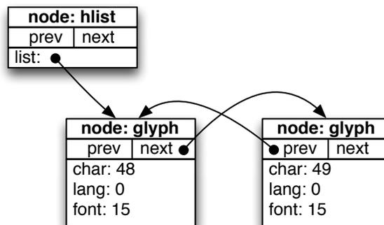
The *list* entry of the hlist (hbox) points to the *node list* starting with the digit 0. The idea for our second approach is to create a node list that represents the vertical bars and gaps (rule and kern nodes) and digits. We create a few more helper functions as well as the new main function:
